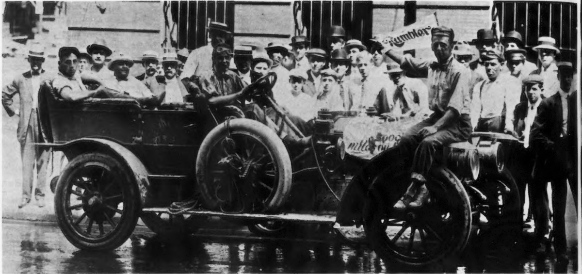
A typical scene of an early day endurance run to confirm a car's durability. This one is heralding a 5000 mile trip in a Rambler. Note the "spoon" support for the horn bulb behind the driver's elbow for rapid action. Photo submitted by Rodger Abbott of Pasadena, Cal.
